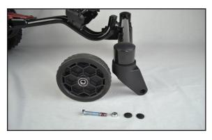
**Step 5:** Adjust the torque for normal rotation. The wheel should achieve roughly 5 rotations on a single spin. Replace caster wheel caps.
