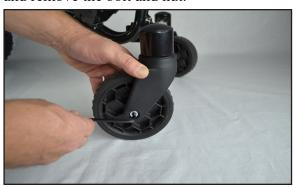
**Step 4:** Install the replacement caster wheel with the 6 mm hex bolt and nut.
